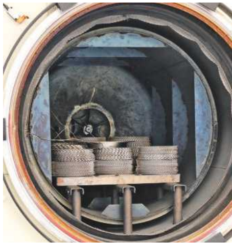
No, not an industrial washing machine, but an oven for annealing the blades
